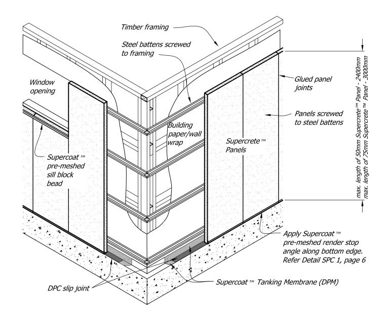
**NOTE:** The Supercrete ™ Distributor determines the correct batten spacing using wind and earthquake load information supplied by the building owner on the design documents.
